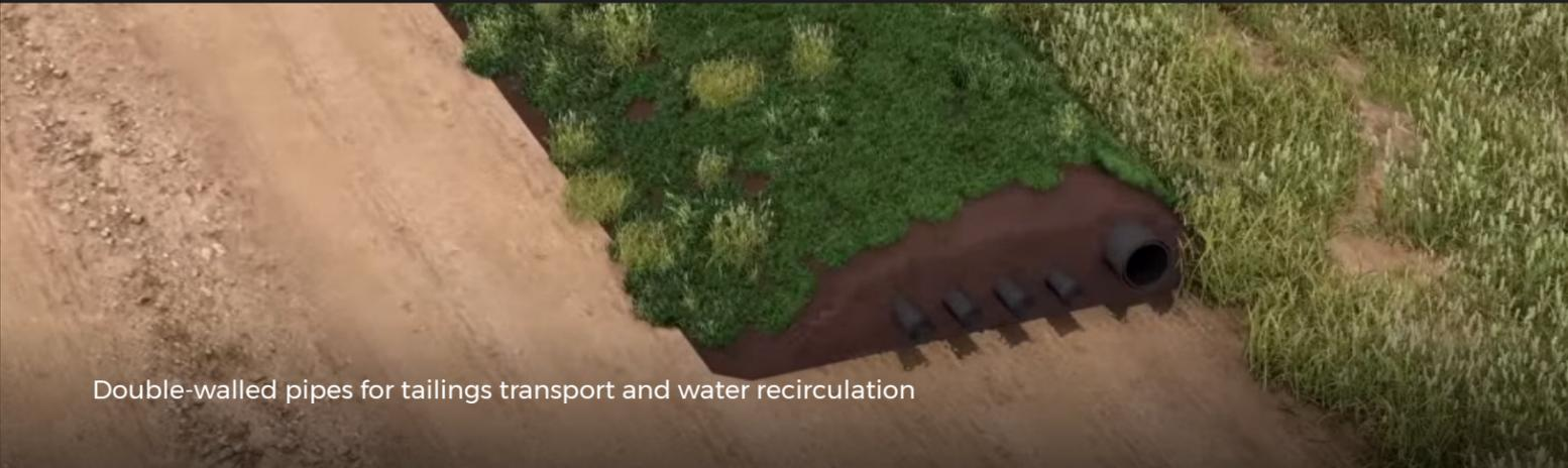
Double-walled pipes for tailings transport and water recirculation
